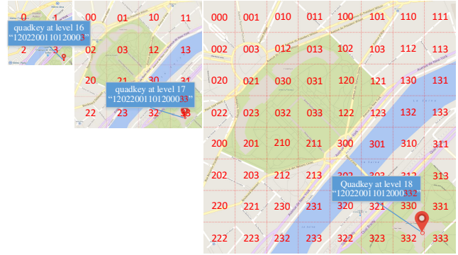
Figure 2: Hierarchical map gridding based on the Tile Map System, and the mapping of a location (the Eiffel Tower) into grids at level 16-18, whose quadkeys are annotated.
