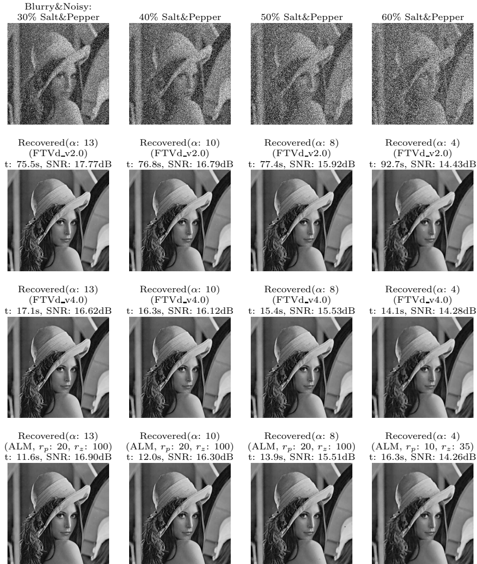
FIGURE 3. TV- L^1 restoration from 7 \times 7 sized Gaussian blur with salt-and-pepper noise from 30% to 60% (image size 512 \times 512 ).
