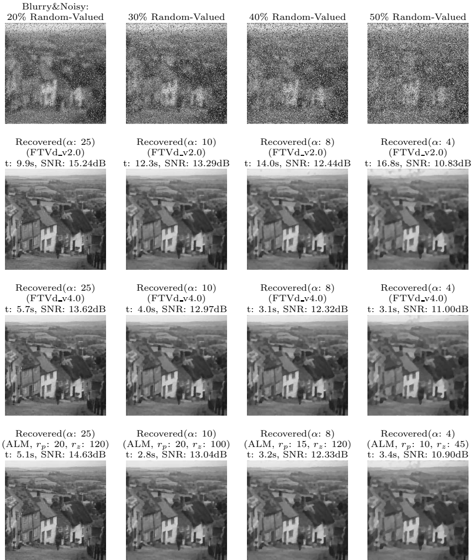
FIGURE 4. TV- L^1 restoration from 7 \times 7 sized Gaussian blur with random-valued noise from 20% to 50% (image size 256 \times 256 ).
