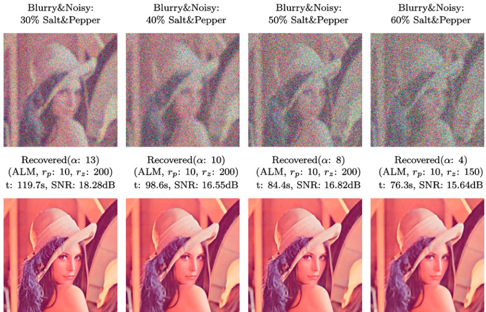
Fig. 1. Recovered from blur with salt-and-pepper noise from 30% to 60%. The blur operator is the one in (19). All the results are obtained by using the MTV- L^1 model (15) with different numerical solvers (image size: 512 \times 512 ).
