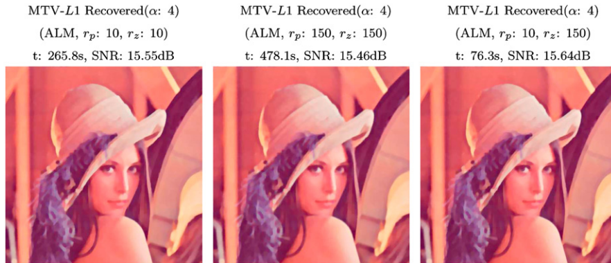
Fig. 4. MTV- L^1 restoration from blurry image with 60% salt-and-pepper noise: a better computational efficiency with comparable restoration result (similar SNRs) is achieved by letting r_p \neq r_z .
