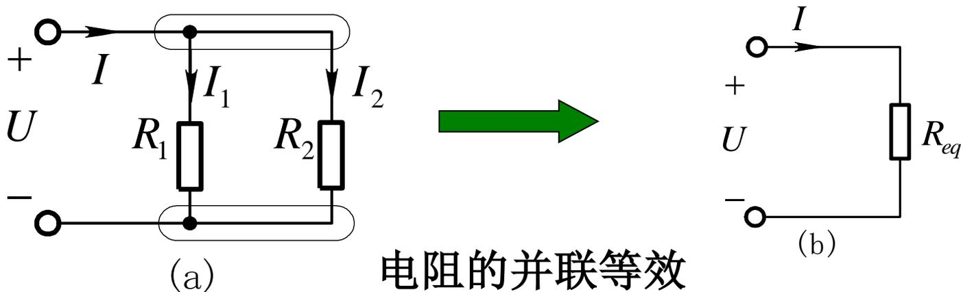
$$I = I_1 + I_2 = \frac{U}{R_1} + \frac{U}{R_2} = (G_1 + G_2)U$$
