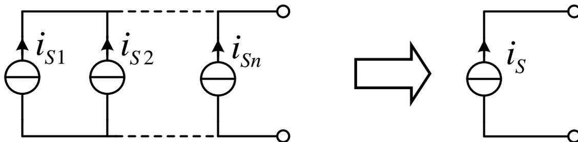
$$i_S = i_{S1} + i_{S2} + \dots + i_{Sn} = \sum i_{Sk} \quad (\text{注意参考方向})$$
