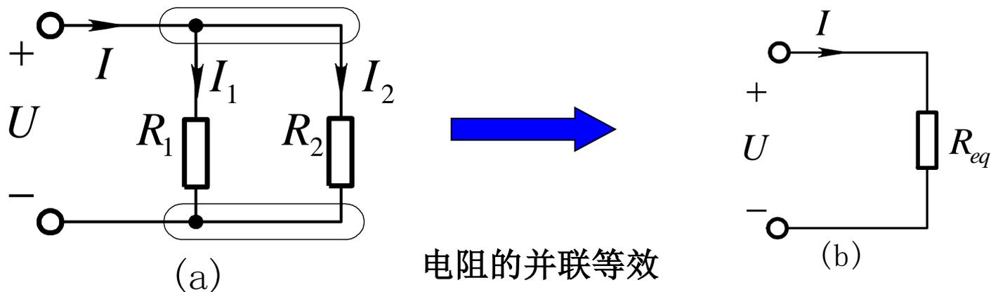
$$I_1 = G_1 U = \frac{G_1}{G_1 + G_2} I = \frac{R_2}{R_1 + R_2} I$$
