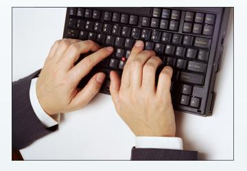
Input is any data or instructions that are used by a computer. Input devices are hardware used to translate words, sounds, images, and actions that people understand into a form that the system unit can process. These include keyboards, pointing, scanning, image capturing, and audio-input devices.
