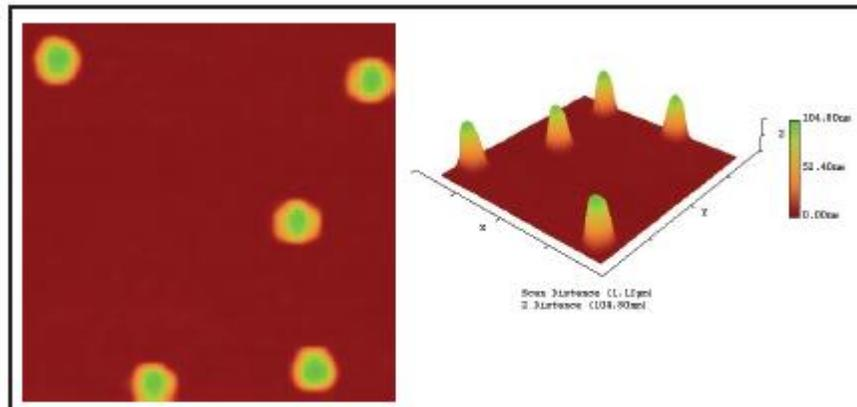
Figure 2: Left: NIST traceable polystyrene microspheres from Duke Scientific scanned with the NANO-RP™. Mean  $\varnothing$  of microspheres is 102nm. Scan size is  $1\mu\text{m} \times 1\mu\text{m}$ . Right: 3D view of  $1 \times 1\mu\text{m}$  scan of calibrated spheres.
