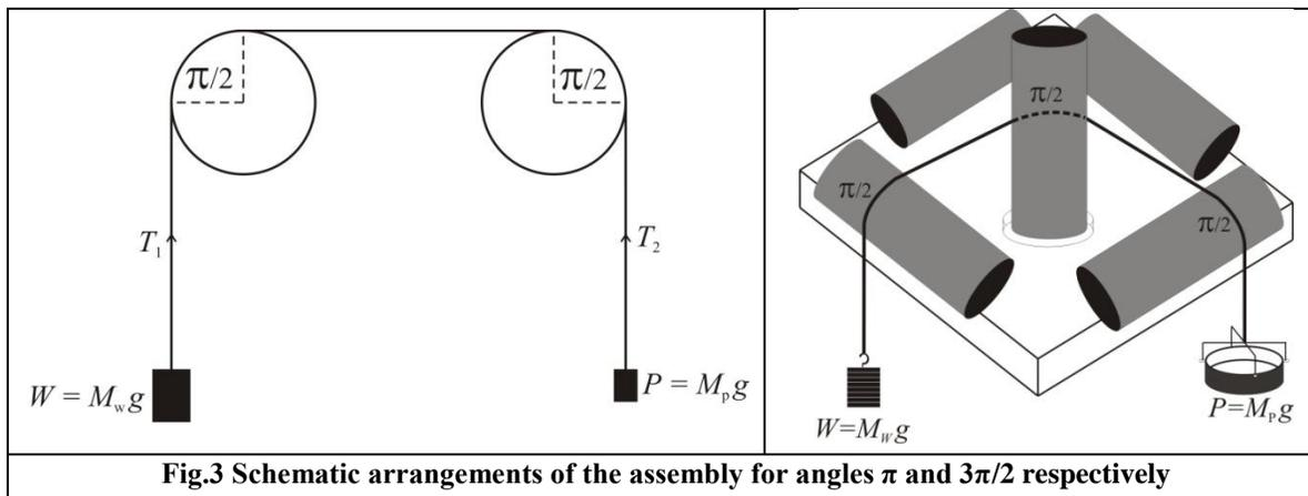
The minimum value of angle  $\theta$  is obtained when the cord passes over two parallel rods without making any contact with the central post (Fig.3). By winding the cord around the vertical post and shifting the position of the effort the angle  $\theta$  can be changed by steps of  $\pi/2$ . The load  $M_w$  should be suspended from the pipe to which the ruled acrylic plate is mounted.
