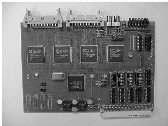
Fig. 2. Photograph of VME Field Programmable Gate Array (FPGA) module developed for prototyping of logic design.
