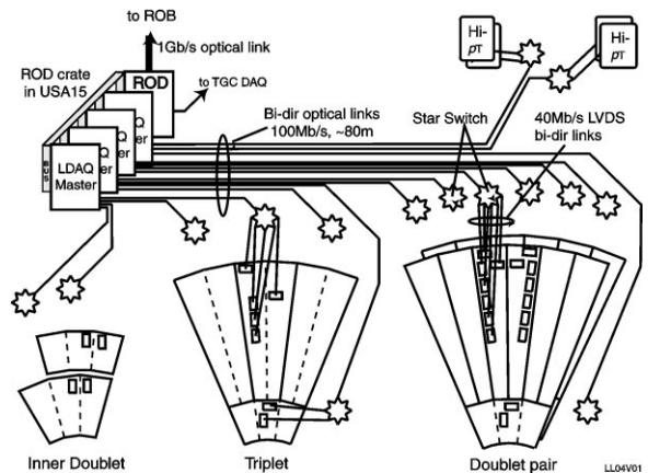
Fig. 1. Schematic diagram of the readout system architecture for the ATLAS TGC.
