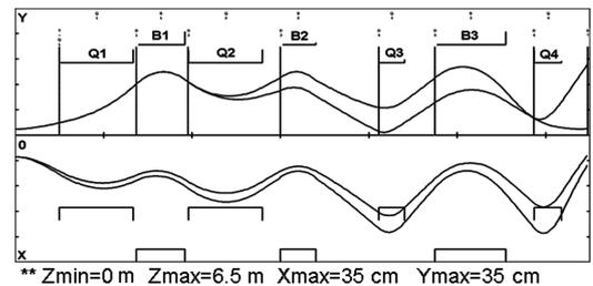
**Fig.6** Horizontal and vertical envelopes for the surface muon beam in transport system
