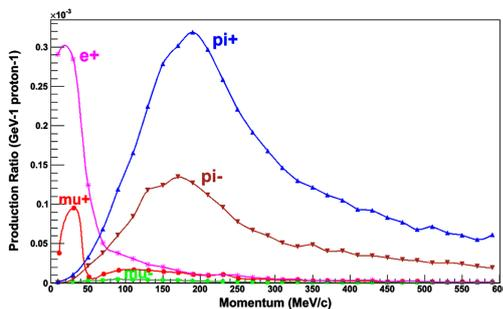
**Fig.2** Production ratio of secondly particles for a graphite target of 15 mm in height and 80 mm in length (color online)
