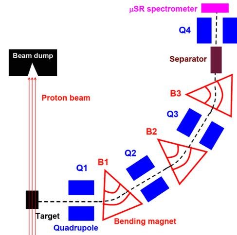
**Fig.5** Layout of the simple surface muon beamline
