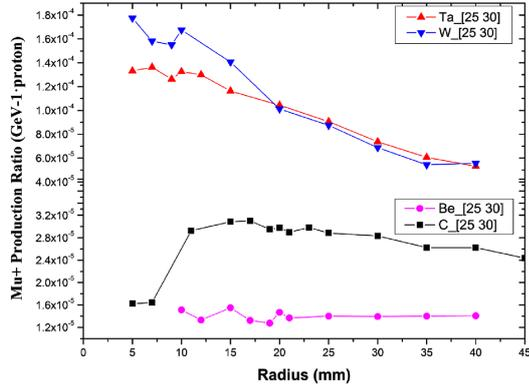
**Fig.3** Surface muon production ratio vs. target radius for a graphite target of 80 mm in length: result using Geant4 (color online)
