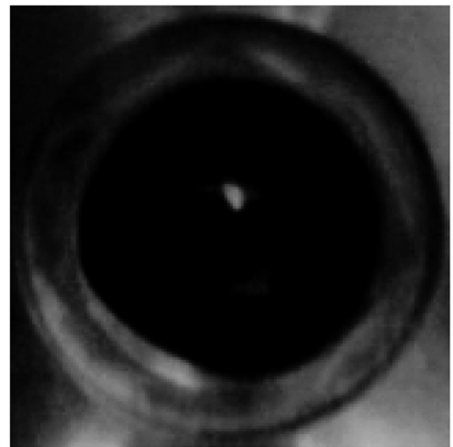
Fig. 4. The practical profile of the electron beam spot in our pulsed positron beam device.
