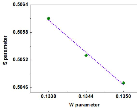
Fig.5 The variation of S- versus W-parameter for Cu<sub>2</sub>Te samples.
