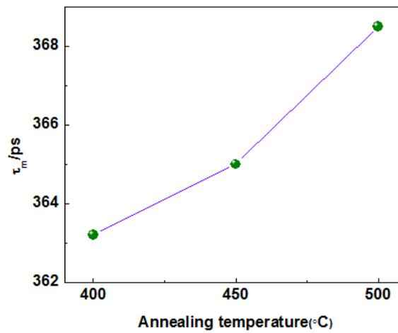
Fig.2 Average lifetime as a function of the annealing temperatures for Cu<sub>2</sub>Te samples.
