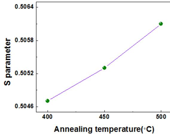
Fig.3 The S-parameter as a function of the annealing temperatures for Cu<sub>2</sub>Te samples.
