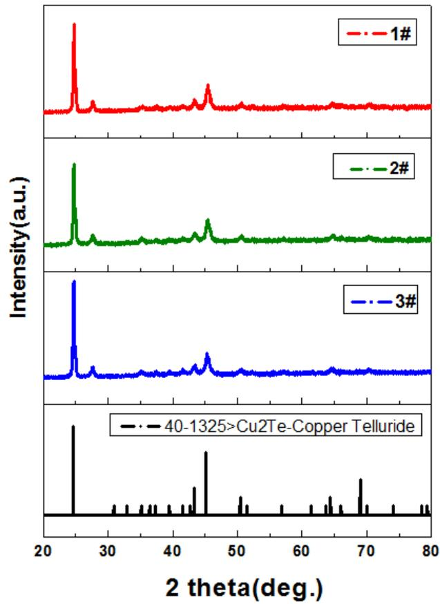
Fig.1 XRD spectra of the Cu<sub>2</sub>Te samples.
