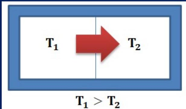
$$dS_1 = \frac{-\delta Q}{T_1}, \quad dS_2 = \frac{\delta Q}{T_2}$$
