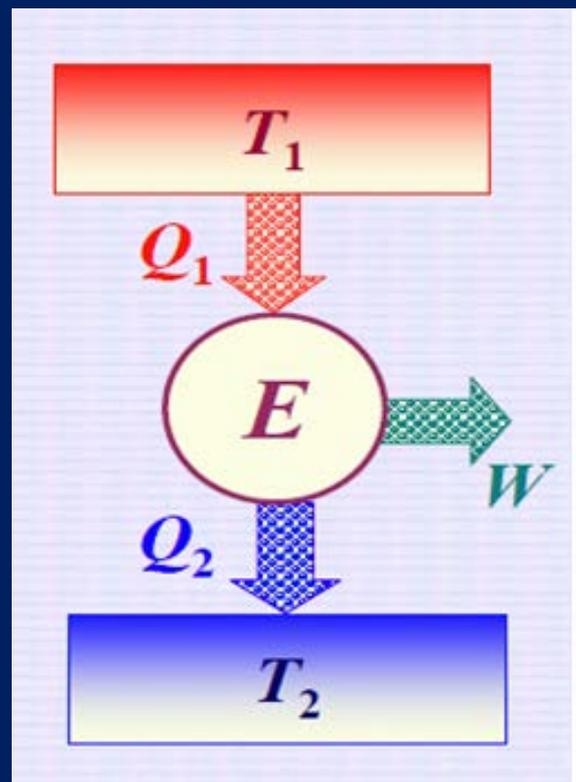
$$\eta = 1 - \frac{Q_2}{Q_1} \leq 1 - \frac{T_2}{T_1} \quad \left\{ \begin{array}{l} = : \text{对应可逆机} \\ < : \text{对应不可逆机} \end{array} \right.$$
