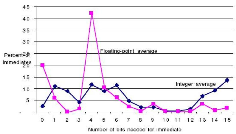
The distribution of immediate values. About 20% were negative for CINT2000 and about 30% were negative for CFP2000. These measurements were taken on a Alpha, where the maximum immediate is 16 bits, for the spec cpu2000 programs. A similar measurement on the VAX, which supported 32-bit immediates, showed that about 20% to 25% of immediates were longer than 16 bits.
