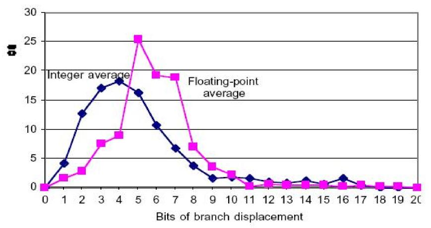
Alpha Architecture with full optimization for Spec CPU2000, showing the average of integer programs(CINT2000) and the average of floating-point programs (CFP2000) 建议: shorter offsets are the most common
