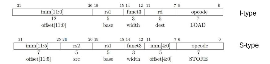
Load and store instructions transfer a value between the registers and memory. Loads are encoded in the I-type format and stores are S-type. The effective address is obtained by adding register rs1 to the sign-extended 12-bit offset. Loads copy a value from memory to register rd. Stores copy the value in register rs2 to memory.
