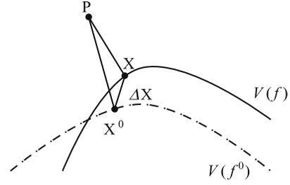
Fig. 1. Estimation of foot-point on an active implicit curve
