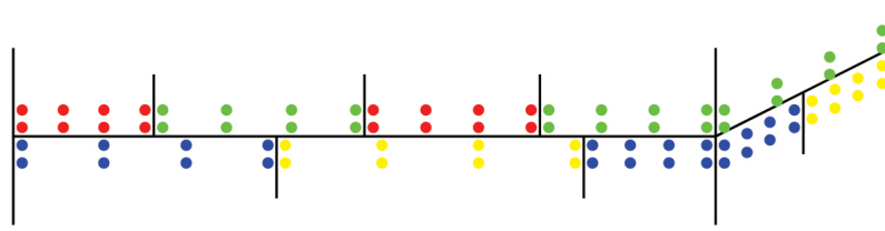
Fig. 4: Bézier ordinates in every cell near a c-face ( m = n = k = 3, \alpha = \beta = \gamma = 1 ).
