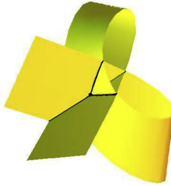
Fig. 3. Rational ruled surface with an order 3 singular point as the intersection of two order 2 self-intersection curves.
