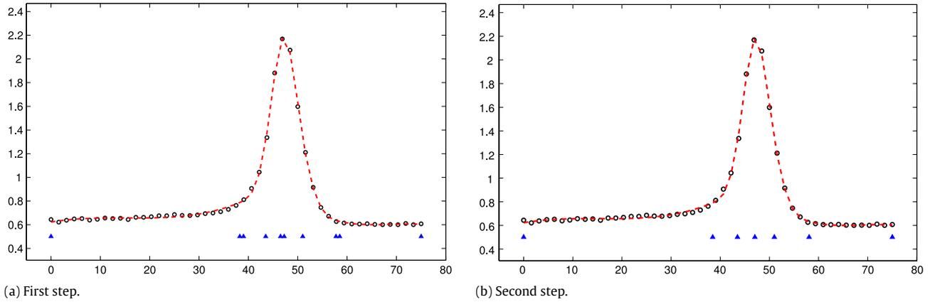
**Fig. 5.** Approximation of Titanium heat data by our algorithm with  $MSE = 0.014128$ . The circles are sample points and the dashed line is the approximated spline by our method. The triangles in (a) and (b) are marked for the knots optimized by the first step and the second step respectively.
