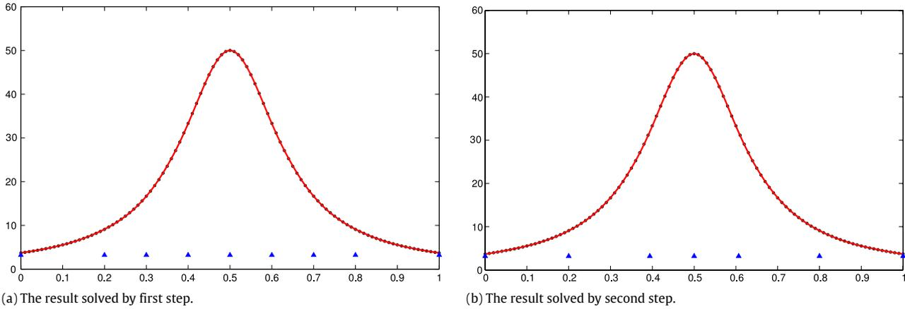
**Fig. 2.** Workflow of knot calculation. (a) The blue triangles are marked for the active knots of the approximated B-spline (red curve) solved by first step. (b) The knots (blue triangles) and the corresponding approximated B-spline (red curve) obtained by second step.
