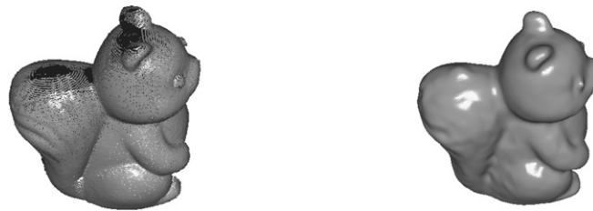
Fig. 10. Reconstruction of incomplete data. Left: the incomplete Squirrel data with holes on the head and the body. Right: the reconstructed Squirrel with holes filled.
