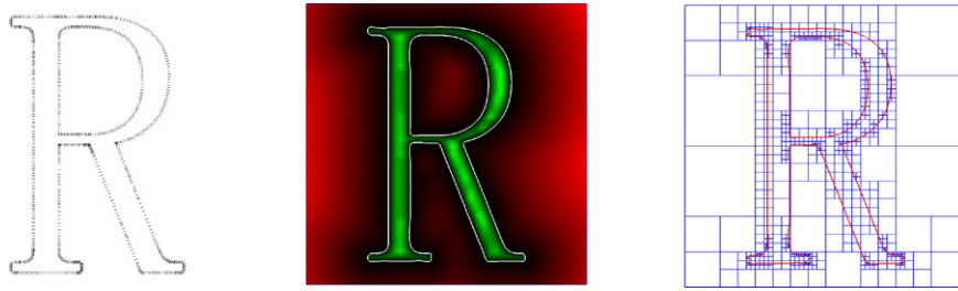
Fig. 3. Left: a set of points with normals from letter 'R'; Middle: the signed distance function and the zero level set; Right: the hierarchical T-mesh and the reconstructed implicit PHT-spline curve.
