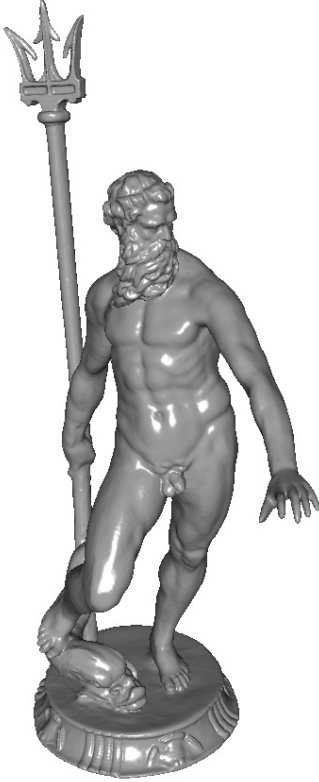
Figure 8: Reconstruction of Neptune model with 2,003,932 points.
