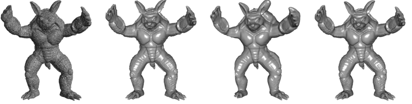
Figure 9: Reconstruction of data with noisy normals(60 degrees rotational deviation in the origin normal direction) by different methods. From leftmost to rightmost are: Armadillo model with noisy normals, MPU reconstruction, Poisson reconstruction and our result.
