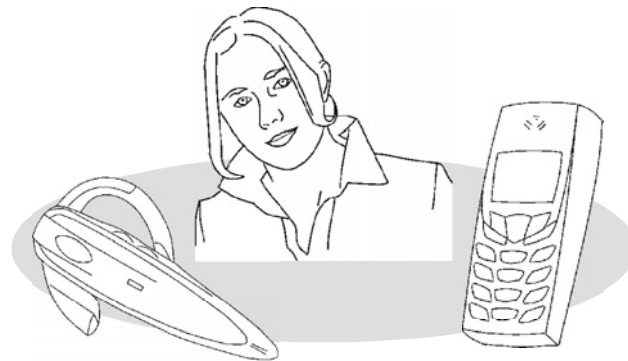
Figure 9.4 A personal-area bubble comprises a collection of consumer electronic devices that typically communicate over a relatively short distance.
