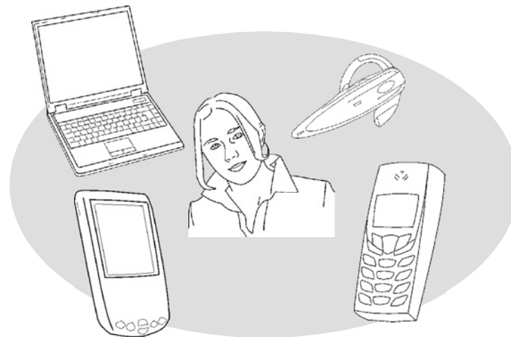
Figure 3.3 A personal-area network comprises the collection of electronic devices that typically communicate over a relatively short distance. In this example, a user has a Bluetooth-enabled headset along with a cellular phone, notebook and PDA.
