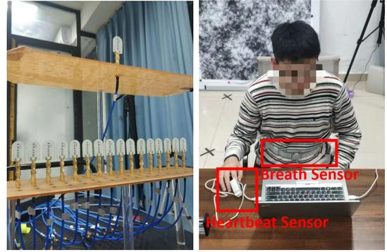
(a) Antenna Configuration (b) Static Human Configuration
