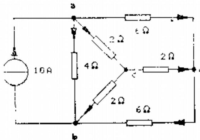
$$R_{ab} = \frac{R_a R_b + R_b R_d + R_a R_d}{R_d} = \frac{2 \times 2 + 2 \times 2 + 2 \times 2}{2} = 6\Omega$$
