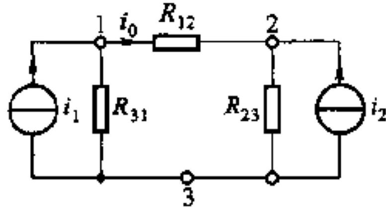
$$\left. \begin{aligned} u_{13} &= \frac{R_{31}(R_{12} + R_{23})}{R_{12} + R_{23} + R_{31}} i_1 + \frac{R_{23}R_{31}}{R_{12} + R_{23} + R_{31}} i_2 \\ u_{23} &= \frac{R_{23}R_{31}}{R_{12} + R_{23} + R_{31}} i_1 + \frac{R_{23}(R_{12} + R_{31})}{R_{12} + R_{23} + R_{31}} i_2 \end{aligned} \right\} \quad (2)$$
