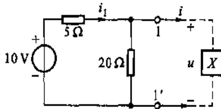
$$\begin{aligned} 10 &= 5i_1 + u \\ u &= 20(i_1 - i) \end{aligned}$$
