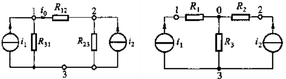
$$\left. \begin{aligned} R_1 + R_3 &= \frac{R_{31}(R_{12} + R_{23})}{R_{12} + R_{23} + R_{31}} \\ R_3 &= \frac{R_{23}R_{31}}{R_{12} + R_{23} + R_{31}} \\ R_2 + R_3 &= \frac{R_{23}(R_{12} + R_{31})}{R_{12} + R_{23} + R_{31}} \end{aligned} \right\} \Rightarrow \left. \begin{aligned} R_1 &= \frac{R_{31}R_{12}}{R_{12} + R_{23} + R_{31}} \\ R_2 &= \frac{R_{12}R_{23}}{R_{12} + R_{23} + R_{31}} \\ R_3 &= \frac{R_{23}R_{31}}{R_{12} + R_{23} + R_{31}} \end{aligned} \right\}$$
