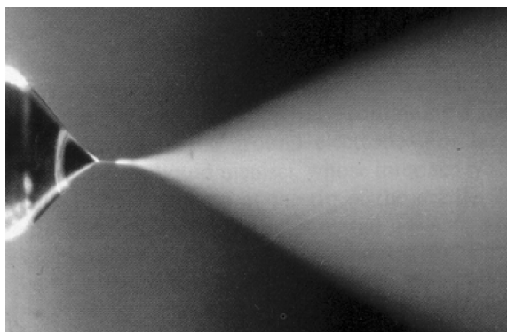
Fig. 3. Cone-jet spraying of methanol containing a small amount of hydrochloric acid [35].
