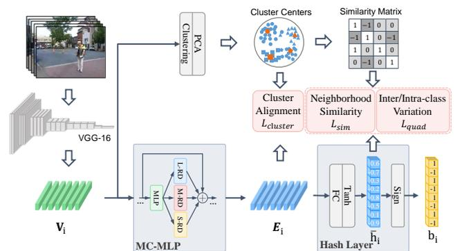
**Figure 1: Overall structure of the proposed MCMSH. The MC-MLP module is designed to learn discriminative video representations by capturing multiple granularities of axial contexts. Three kinds of unsupervised learning objectives are developed to optimize the hash code generation.**
