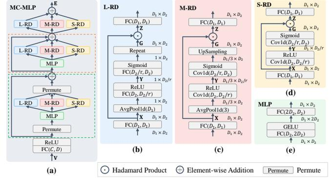
**Figure 2: The schema of the proposed (a) MC-MLP model. It mainly consists of four blocks, i.e., (b) L-RD, (c) M-RD, (d) S-RD and (e) MLP.**
