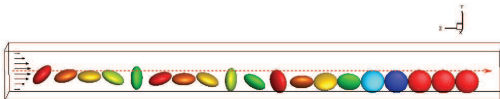
Figure 14: Motion of an oblate ellipsoid inside a square tube Poiseuille flow.
