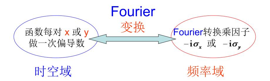
$$a\frac{\partial^2 u}{\partial x^2} + b\frac{\partial^2 u}{\partial x \partial y} + c\frac{\partial^2 u}{\partial y^2} = 0 \qquad -a\sigma_x^2 - b\sigma_x\sigma_y - c\sigma_y^2 = 0$$
