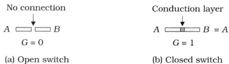
Figure 3.11 Simplified operational view of an nFET 栅信号G决定了在漏区与源区之间是否存在导电区
