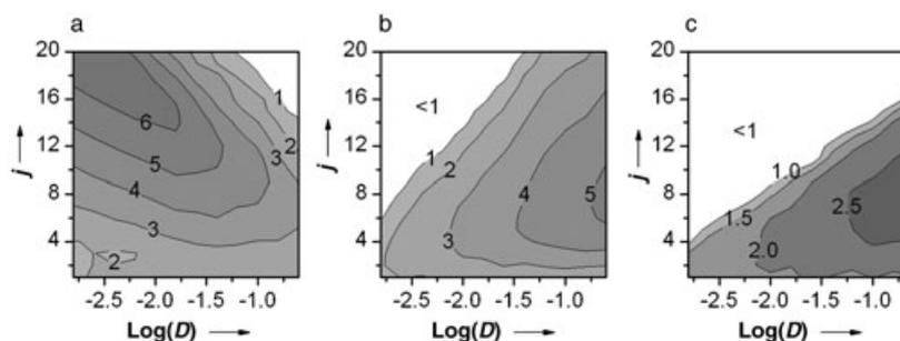
**Figure 2.** SNR plots for different cases from Figure 1. a) Global noise is used. The results shown here are for uncorrelated noises, but same qualitative results are obtained for correlated ones; b)  $r_0=1.03$ ; c) two-way coupling. In all three diagrams, the values on the contour lines denote the logarithm of the SNR.
