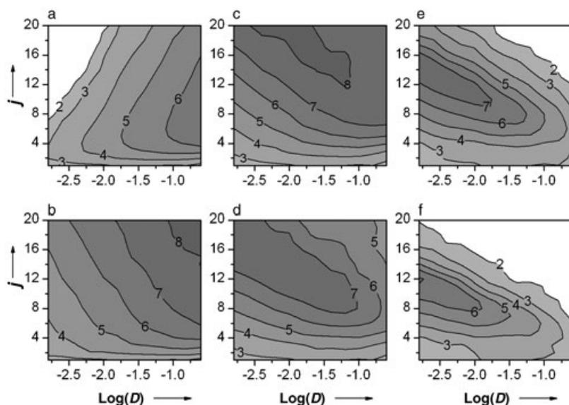
**Figure 3.** SNR plot for different coupling strengths. From a) to f), the coupling constant  $C$  is 0.2, 0.3, 0.4, 0.5, 0.6, and 0.7, respectively. It is clear that  $C=0.3$  is optimal for the amplified propagation of the NIO.
