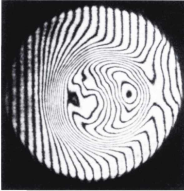
Fig. 4.17. Interferometric image of a \theta pinch [courtesy F. Jahoda (1985), private communication] showing the circular plasma compressed away from the outer low-density regions in which the fringes are straight.
