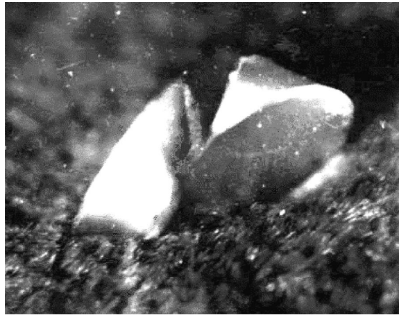
Fig. 6. Photograph of a broken specimen under dynamic compression/shear loading.
