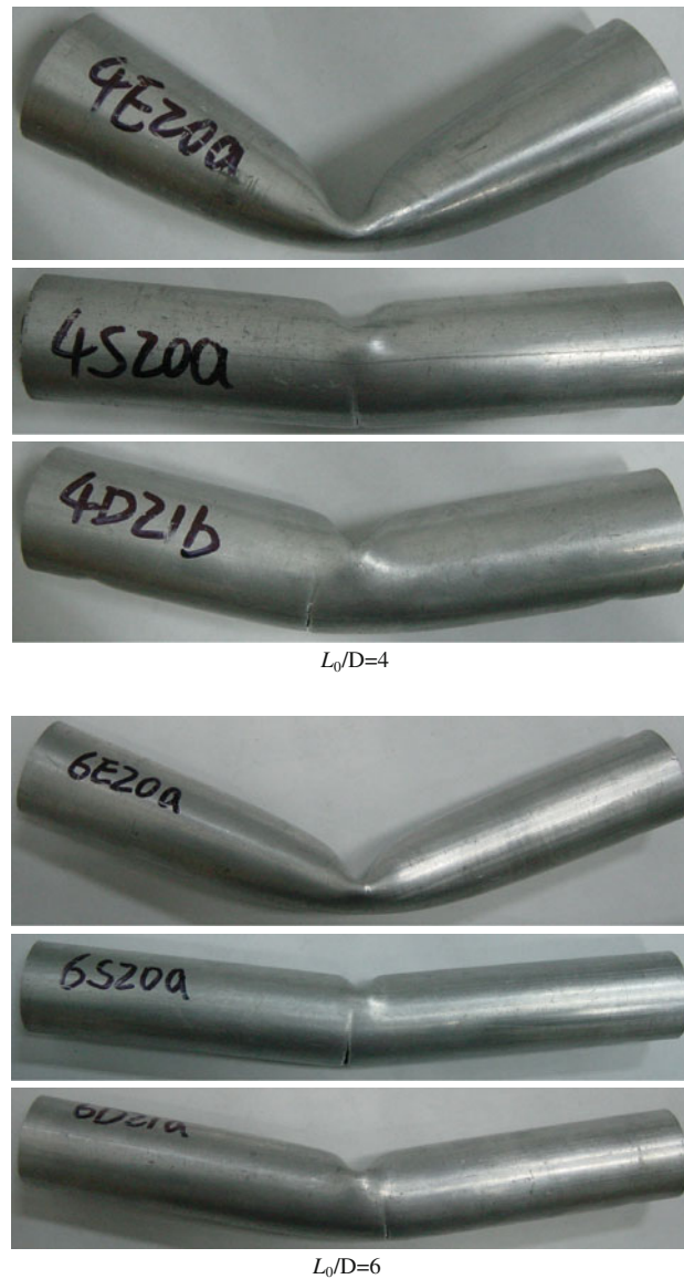
Fig. 6 Final deformation of different tube structures
