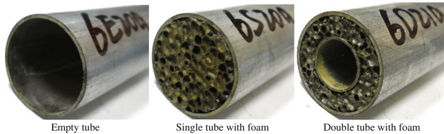
Fig. 3 Sections of different tube arrangements
