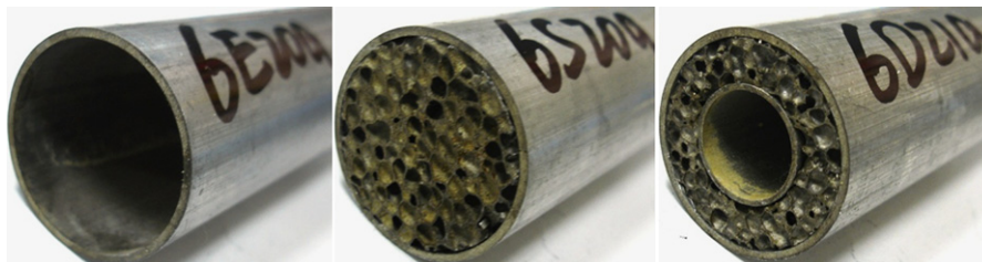
Fig. 5. Section view of empty and foam-filled structures.
