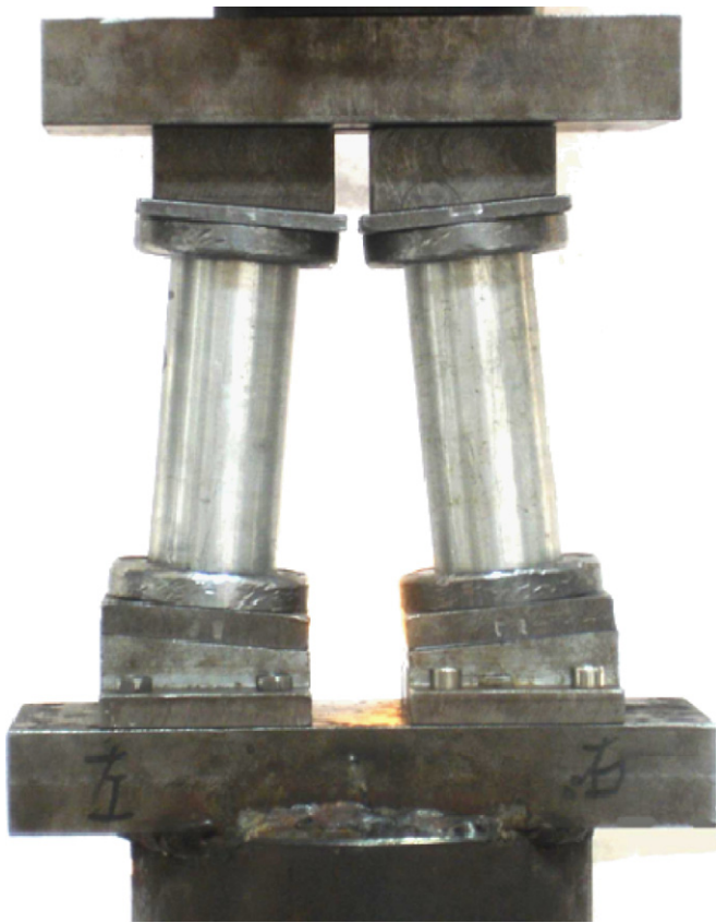
Fig. 1. The oblique loading rig used in test of tubular structures.
