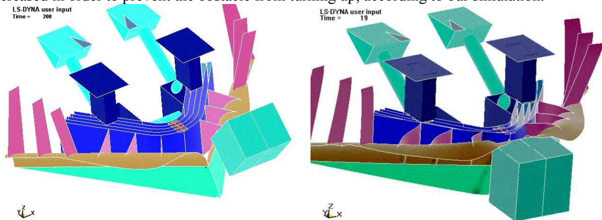
Fig. 6. A train with a cowcatcher crashes an obstacle at v = 10 m/s (left) or v = 50 m/s (right).
