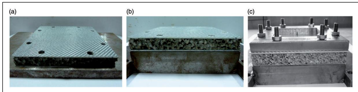
**Figure 2.** Photographs of the boundary conditions: (a) placed on the top of a rigid substrate without any clamping device (RS); (b) placed on a specially designed frame with panel edges SS; (c) fully clamped (FF).
