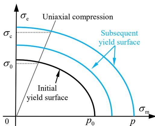
Fig. 1 Yield surfaces for the Deshpande-Fleck foam model.
