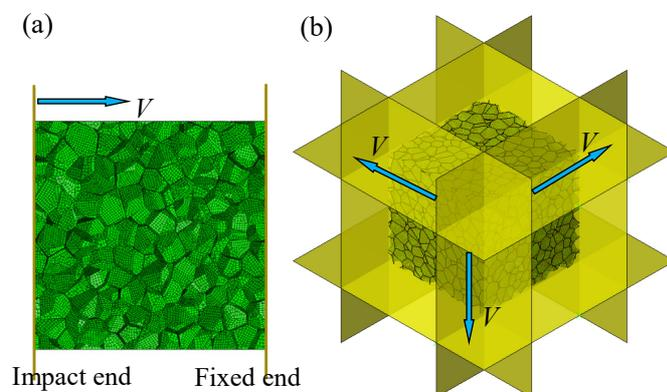
Fig. 2 Cell-based finite element models of (a) uniaxial compression and (b) hydrostatic compression.
