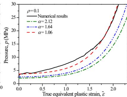
Fig. 4 Predictions of hydrostatic pressure using different value of  $\alpha$ .
