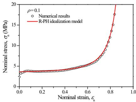
Fig. 3 Quasi-static uniaxial compression stress–strain relation and the fitting by R-PH model.
