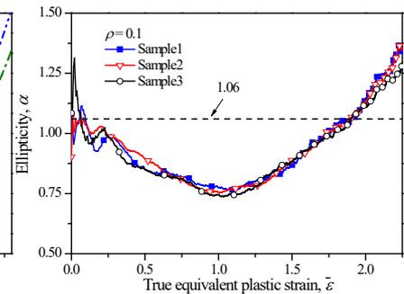
Fig. 5 Ellipticity  $\alpha$  calculated by Eq. (9).
