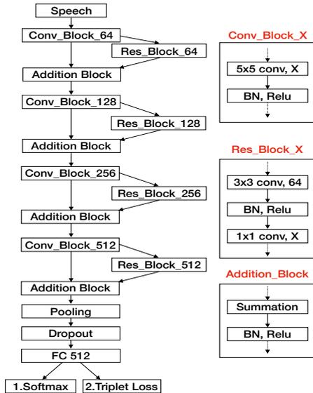
Figure 3: The architecture of the residual CNN i-vector model.
