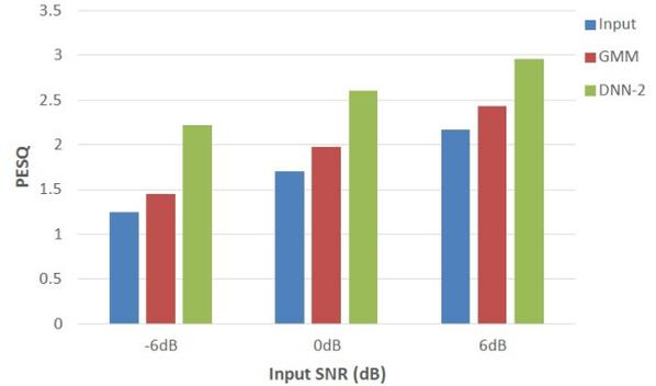
Figure 7: Separation performance (PESQ) comparison of different approaches averaged across all 34 testing target speakers.
