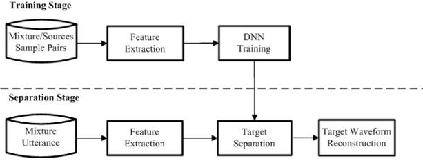
Figure 1: Development flow for speech separation system.
