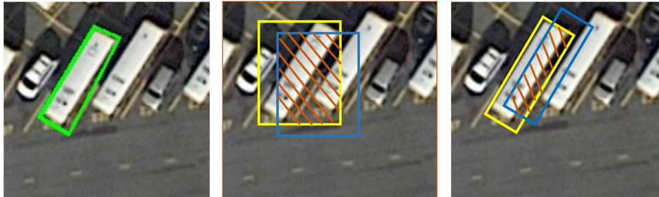
Fig. 6. The intersection over union (IoU) computation of RCR-CNN. From left to right: the quadrangle label, the calculated IoU on the HBB in the first R-CNN stage, and the calculated IoU on the rotated bounding box in the second R-CNN stage (the shaded part is the intersection area).
