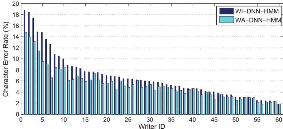
Fig. 6. Performance comparison of WI-DNN-HMM and WA-DNN-HMM with  $K=1000$  on the test set of all 60 writers.
