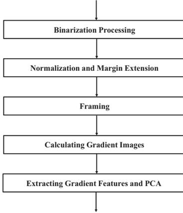
Fig. 2. The procedure of feature extraction.
