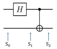
The input state is  $|00\rangle$ , which is stabilized by  $S_0 = \langle IZ, ZI \rangle$ . Give the generators of the stabilizers describing the state after the Hadamard  $S_1$  and after the controlled-NOT gate  $S_2$ . Work this out by using the fact that U acting on a state stabilized by S produces a state stabilized by  $USU^{\dagger}$ .
