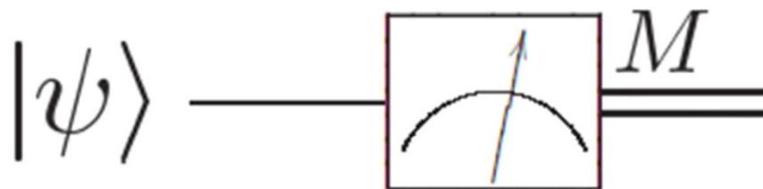
Figure 1.10. Quantum circuit symbol for measurement.
