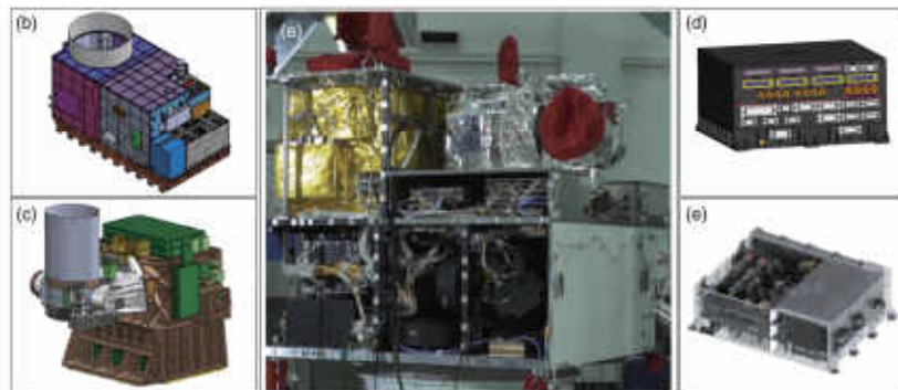
FIG. 18. Full view of the Micius satellite and the main payloads. (a) Photograph of the Micius satellite prior to launch. (b) Transmitter 1 for QKD, entanglement distribution, and teleportation. (c) Transmitter 2, especially designed for entanglement distribution. (d) Experimental control box. (e) Entangled-photon source.
