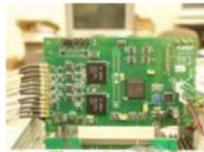
PCI interface high-speed electronics boards for Alice (left) and Bob (right).
