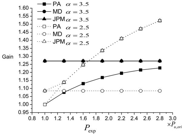
Fig. 2. The energy saving gain of three schemes as a function of  $P_{exp}$ . ( $\lambda_{m,max} = 4 \times 10^{-6} m^{-2}$ )
