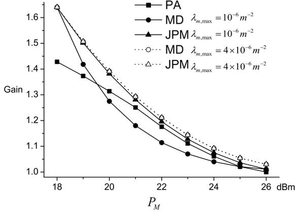
Fig. 1. The energy saving gain of three schemes as a function of  $P_M$ .
