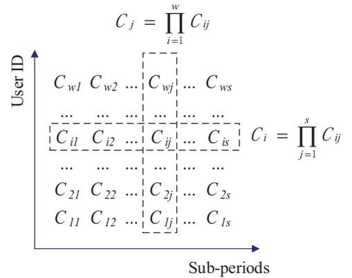
Fig. 3. Aggregator's Cached Data and Two Aggregation Operations
