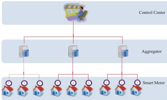
Fig. 1. Network Model for Smart Grid
