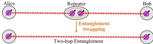
Fig. 2. Performing a swap operation to establish a two-hop entanglement connection between two distant quantum end nodes.
