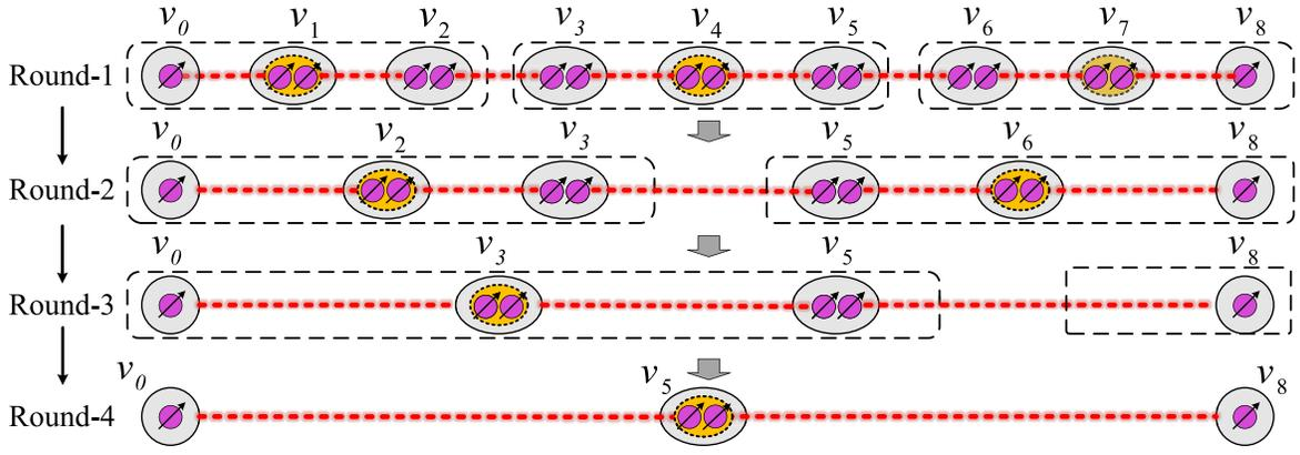
Fig. 8. Remote entanglement distribution achieved by segment-based method.
