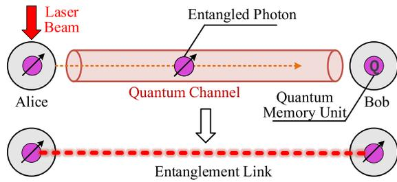
Fig. 1. The implementation of entanglement generation between adjacent quantum nodes based on single-atom excitation scheme.
