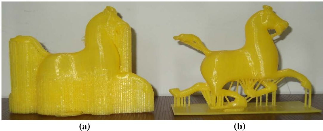
Figure 2: Extrusion-type (FDM) 3D printers need to add extra supporting structures to print the objects. (a) shows the printed result with supporting structure generated by the naive method in commercial software; and (b) shows the printed result with supporting structure generated by our method. It is seen that our method needs much less material used in the supporting structures.
