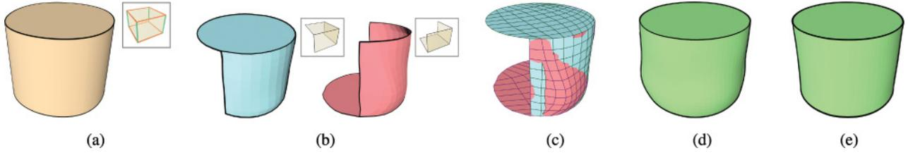
Fig. 3. Given subdivision surface with control mesh (a), the results of sparse representations on individual charts (b), the surface's appearance in overlapping regions (c), the result of a manifold (d) by simple blending, and the obtained surface (e) by compatible sparse representation.
