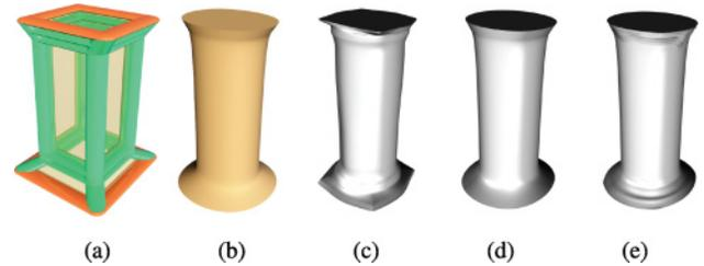
Fig. 9. Manifolds constructed with different sparsity parameters. (a) Input control mesh with  $C^0$  constraints on the edges in red. (b) The limit subdivision surface with sharp features. (c-e) Manifolds constructed by our approach with  $\delta = 5, 25, 55$ , respectively.
