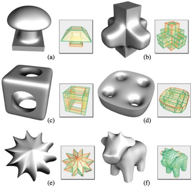
Fig. 8. Examples of manifolds constructed by our approach to approximate the subdivision surfaces with given control meshes in the lower right.  $C^0$  constraints shown in red are enforced to create sharp features in the subdivision surfaces.
