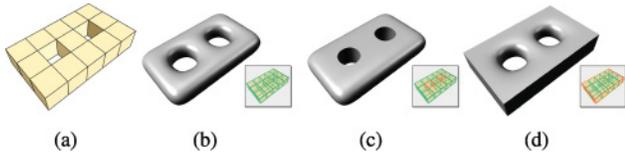
Fig. 7. (a) Control mesh. (b-d) Manifolds constructed by our approach to approximate the subdivision surface with various  $C^0$  constraints on the edges (shown in red).
