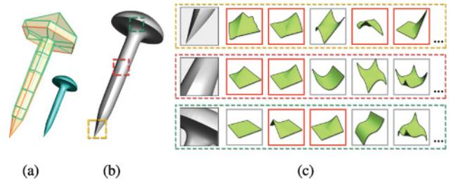
Fig. 5. Constructing manifold to approximate subdivision surface. (a) The input control mesh with enforced  $C^0$  features shown in red. (b) The manifold generated by our approach. (c) The close-up views of three parts of sharp features including crease, dart, and cusp. The first five atom functions that are adaptively selected for representing the local features are shown.
