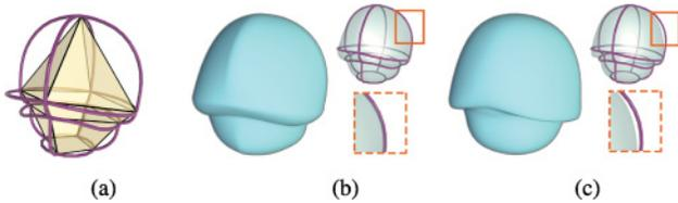
Fig. 15. The fitting of a mushroom like curve network. (a) Illustration of the curve network and domain manifold. The result of our method is shown as (b), and the result using only polynomials is shown as (c). Note that (b) fits better on the curves than (c) with  $C^0$  functions.
