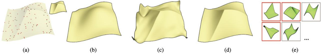
Fig. 2. Given a set of sampling points (100 points in total) from a  $C^0$  surface (a), the obtained fitting surface via polynomials (b), redundant atom functions (c), and sparse representation (d). (e) The first five atom functions ( $C^0$  shape functions in red boxes and polynomials in gray boxes) selected in the sparse representation. The sparsity is set at 25.
