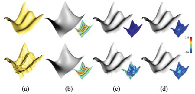
Fig. 4. The results of representing local geometry (a) using least-squares method and sparse representation with fitting error visualized by color map. Approximating results in the fashion of least-squares using polynomials with degree up to 5 (b) and 14 (c); approximating results using sparse representation (d). The input consist of clean data (upper row) and noisy data (lower row).
