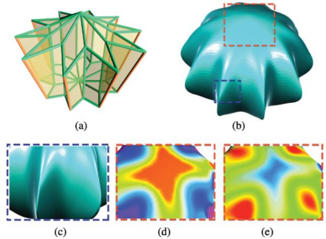
Fig. 12. (a) Control mesh with  $C^0$  constraints shown in red. The top vertex of (a) has a valence of 10. We discard the  $C^0$  atom functions from the dictionary at the chart around this vertex. The manifold surface constructed by our approach is shown in (b). The surface adapts to the sharp features in blue region and is  $C^\infty$  in the red region. (c) Close-up view of the blue region. (d,e) Gaussian curvature and mean curvature of the red region.
