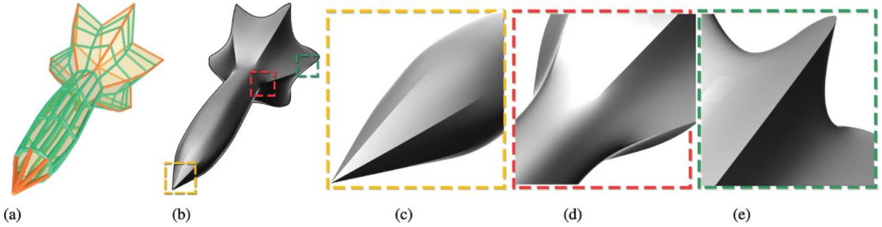
Fig. 6. From a mesh (a), our approach generates a manifold surface (b) approximating its Catmull-Clark subdivision surface. Sharp features are created in the subdivision surface by enforcing  $C^0$  constraints on edges shown in red (a). The constructed manifold (b) approximates various features like crease, dart, and cusp well. The regions in red, green, and blue are zoomed and shown in (c), (d), and (e), respectively.
