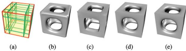
Fig. 11. Manifolds construction approximating subdivision surface with different atom functions. (a) Control mesh. (b) Manifolds generated with only polynomials. (c) Manifolds generated with only shape functions. (d) Manifolds generated with polynomials, spline functions, sine and cosine functions, and shape functions. (e) Manifolds generated with polynomials and shape functions.
