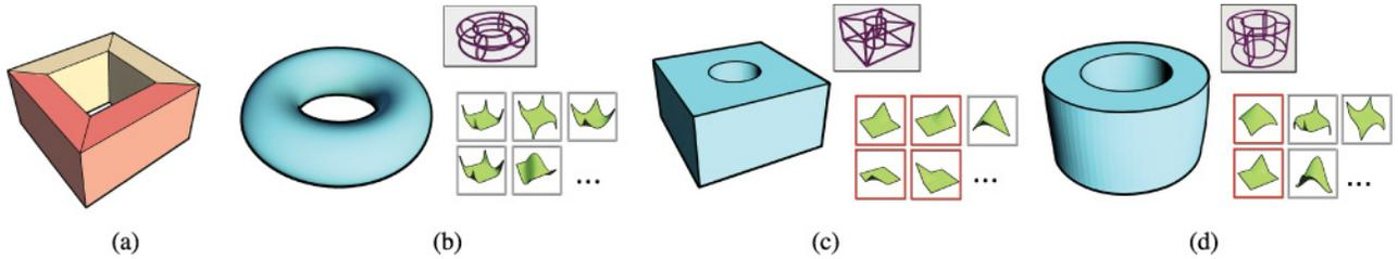
Fig. 14. Generating manifold from different geometries defined on the same domain manifold. (a) The domain mesh. (b-d) Three manifolds created from given curve networks (in the upper right) and the first five chosen atom functions (in the lower right).  $C^0$  shape functions are shown with red frames.
