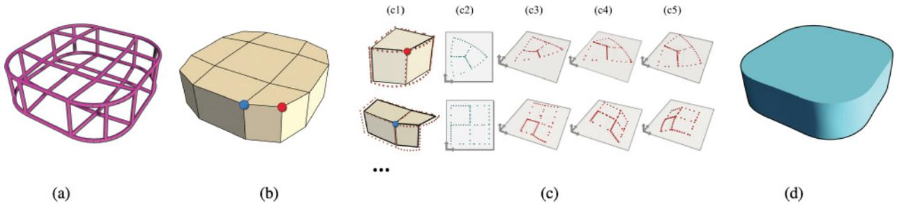
Fig. 13. The procedure for constructing a manifold surface from a given curve network (a). First we use the identified cycle information to build the domain manifold (b). Then we obtain observation data by local parameterization of curves on each chart (c). Finally, the manifold surface (d) is constructed using our approach. (c1) Sampling points on curves. (c2) Local coordinates of samples on individual charts. (c3-c5) The observation data of  $(x, y, z)$ , respectively.
