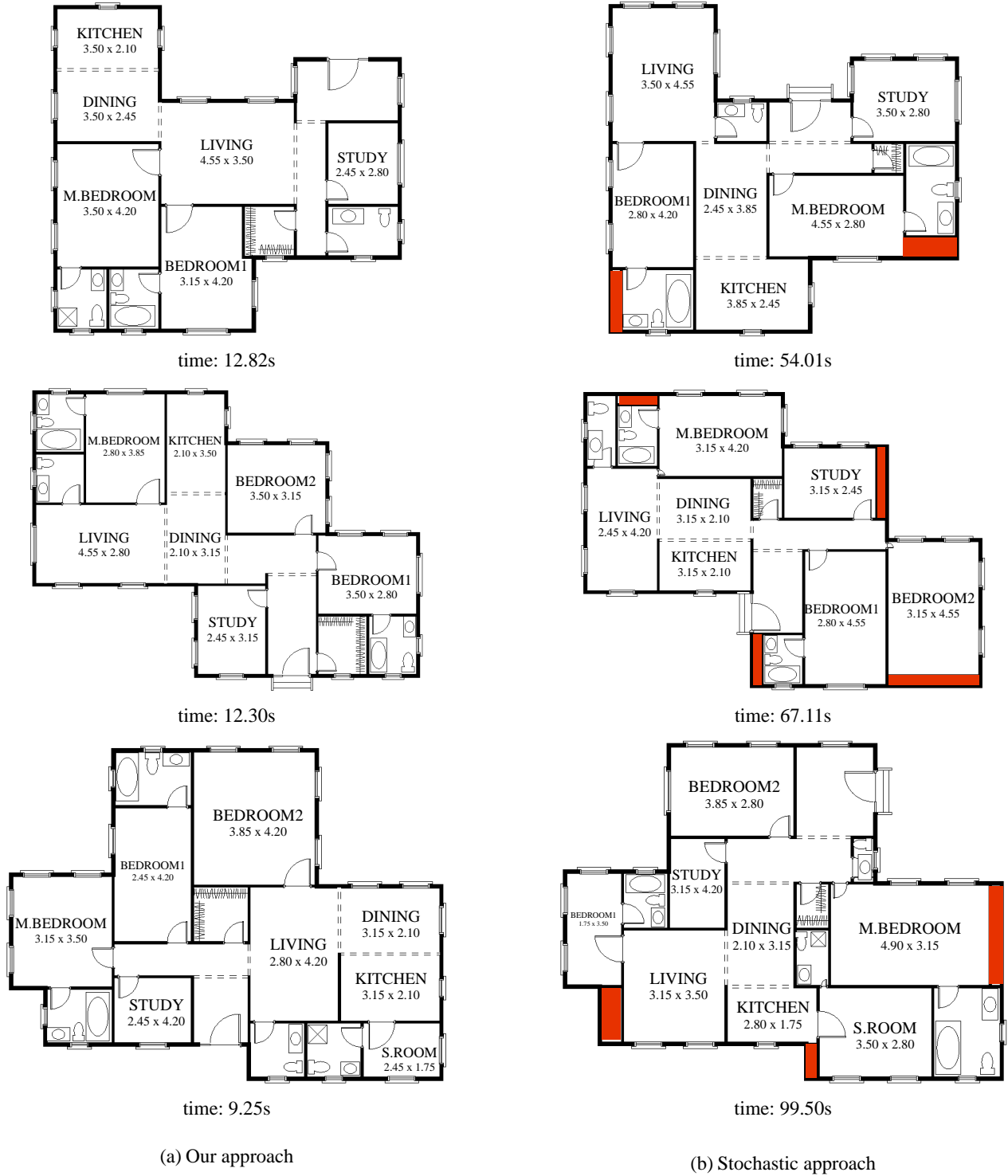
Figure 10: Comparison with the stochastic approach [MSK10]. We show comparisons on rows. Left column: layouts generated by our algorithm. Right column: layouts generated by the stochastic method. Running time of each layout is shown below. Uncovered regions are highlighted in red.
