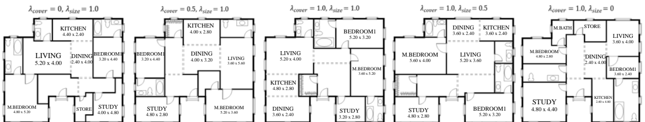
Figure 9: Layouts generated by our algorithm using different weights: \lambda_{cover} and \lambda_{size} . A small \lambda_{cover} gives rise to complex room shapes, while a small \lambda_{size} leads to layouts with large size error.
