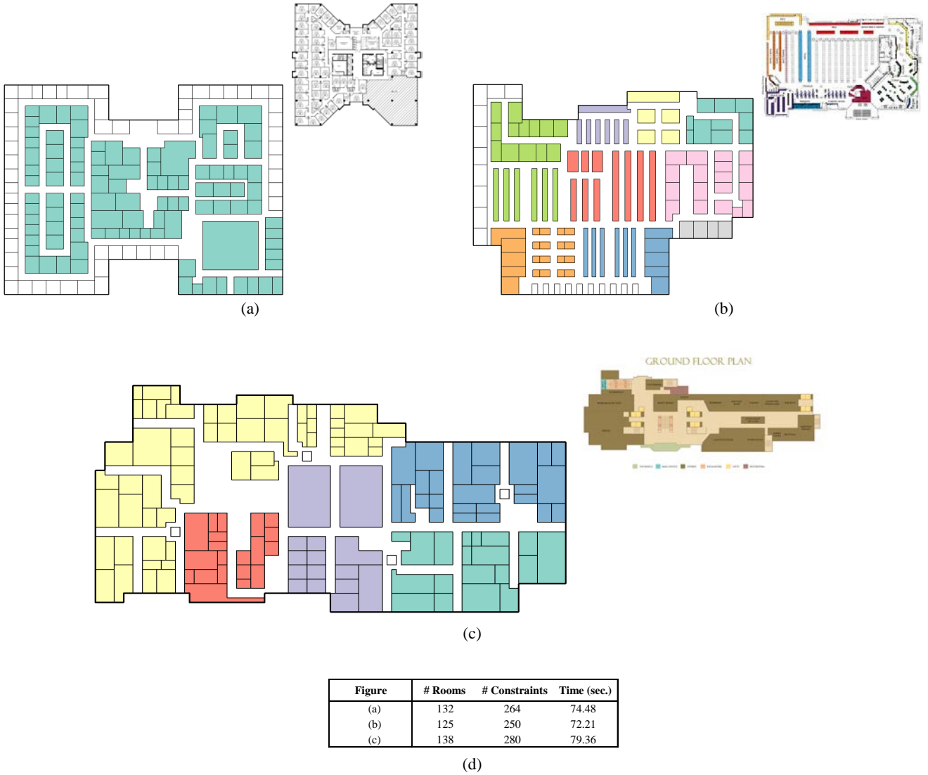
Figure 8: Three large-scale layouts generated by our hierarchical algorithm. (a) office building, (b) supermarket, (c) shopping mall. The boundaries are abstracted from real cases which are shown in the top-right of each layout. (d) shows the number of rooms, the number of constraints, and the running time for each layout.
