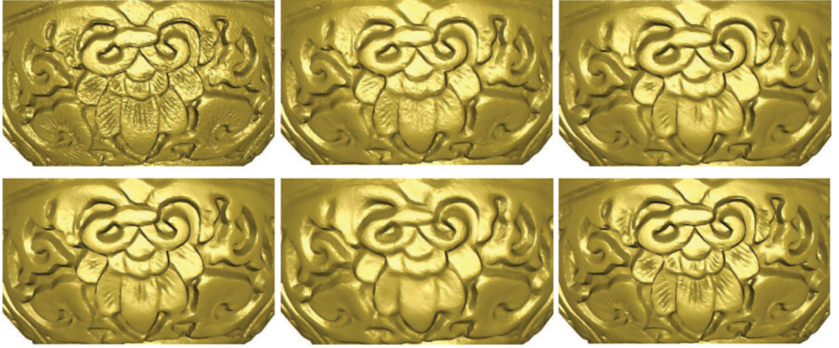
Fig. 14. Denoising of the Decorative pattern embossed model. The left most is the original model, and from middle-topmost to bottom-rightmost: denoising results of Fleishmann et al.'s method ( n = 7 ) [3], Sun et al.'s method ( T = 0.5, n_1 = 3, n_2 = 4 ) [8], Wang et al.'s method ( n_1 = 4, \tau = 0.03, n_2 = 6 ) [11], He and Schaefer's method ( \mu = \sqrt{2}, \alpha = 0.1\bar{\gamma}, \lambda = 0.02\ell_c^2\bar{\gamma} ) [2], and our method ( \sigma_{S1} = 0.35, n_1 = 3, \sigma_{S2} = 0.3, n_2 = 2 ).
