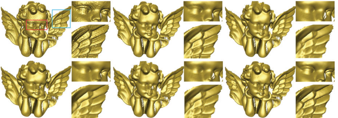
Fig. 13. Denoising of the Angel model. The Leftmost is the original model, and from middle-topmost to bottom-rightmost: denoising results of Fleishman et al.’s method ( n = 15 ) [3], Sun et al.’s method ( T = 0.55, n_1 = 5, n_2 = 10 ) [8], Wang et al.’s method ( n_1 = 5, \tau = 0.05, n_2 = 9 ) [11], He and Schaefer’s method ( \mu = \sqrt{2}, \alpha = 0.1\bar{7}, \lambda = 0.02\ell_c^2\bar{7} ) [2], and our method ( \sigma_{S1} = 0.4, n_1 = 5, \sigma_{S2} = 0.35, n_2 = 4 ).
